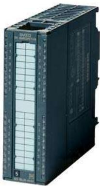
SIMATIC S7-300, Digital output SM 322, isolated, 32 DO, 24 V DC, 0.5A, 1x 40-pole, Total current 4 A/group (16 A/module)
